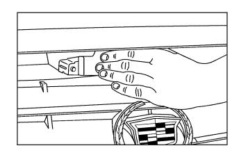
Then go to the front of the vehicle and find the secondary hood release lever. The lever is located under the front edge of the grille near the center. Move the release lever to the side and raise the hood.
